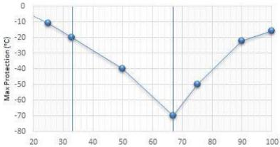
Freezing Protection = Average of Freezing Point (ASTM D1177) and Pour Point (ASTM D97)
