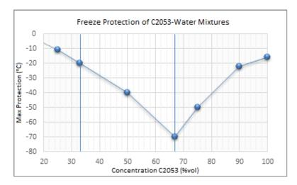
Freezing Protection = Average of Freezing Point (ASTM D1177) and Pour Point (ASTM D97)
